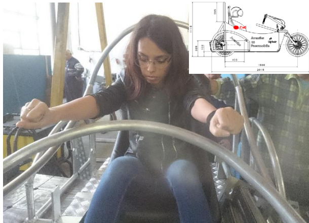
Figure 6. The driver checks the position in conformity with VRAD analysis
