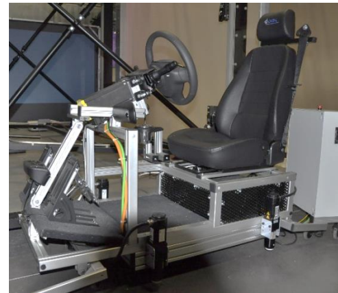
Figure 7. A special driver's seat used in VR immersion (courtesy of Institute Image - ENSAM)
